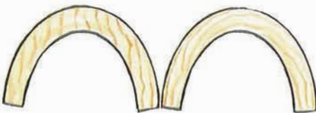
Figure 1: A curve hand-sawn from solid wood (left) usually has significant grain runout, which weakens the piece. The grain lines on a steam bent piece (right), on the other hand, are continuous, making it the stronger alternative.
