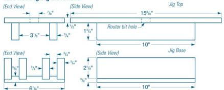
This jig controls the "window" cut on the PVC tubes. Clamp the pipe in place (photo at right). With the router secured to the jig top, align one end of the top to one end of the base. Plunge the bit into the pipe and push the router until the other end of the top aligns with the other end of the base — stop the cut and raise the router.
