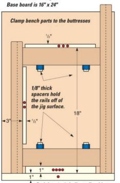
Red dots 1 - 3 indicate fixed buttresses; 4 red dots indicates a spacer.
